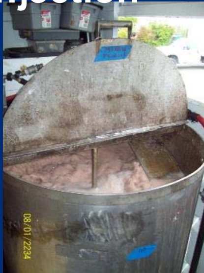
50 gallon batch of agitated 10% by weight gypsum slurry
